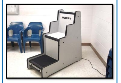
The **BOSS Chair** or **Body ORIFICE Security Scanner** is a non-intrusive scanning system designed to detect small metallic objects such as mobile telephones and weapons, concealed within abdominal cavities and the shin area. This chair is able to detect many items, from large knives to small gun components, which may be hidden by prisoners with the intention of smuggling them into establishments.
